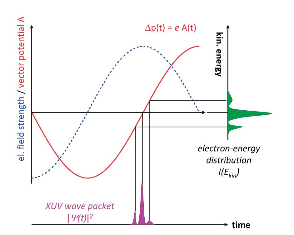
The X-ray pulses from the FEL generate photoions in a gas. The photoelectron energy is thus the X-ray energy minus the binding energy. By introducing an additional electromagnetic terahertz field derived from the pump laser, the photoelectrons "born" inside this field acquire additional energy proportional to the vector potential of the terahertz wave. The final electron energy is thus a function of relative arrival time between the X-ray pulse and the terahertz pulse.
